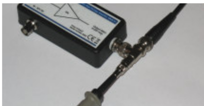
Figure 1. The 10x probe connected for monitoring the output signal
