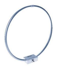
ETS-Lindgren's Model 6511 Passive Loop Antennas have a frequency range of 20 Hz – 5 MHz and are designed for both EMC emissions and EMC immunity tests. All loop antennas can be individually calibrated in accordance with ANSI C63.5, using NIST traceable equipment. By knowing the actual antenna factors and performance characteristics of an antenna instead of typical data, you can more accurately measure field strength in your tests.
