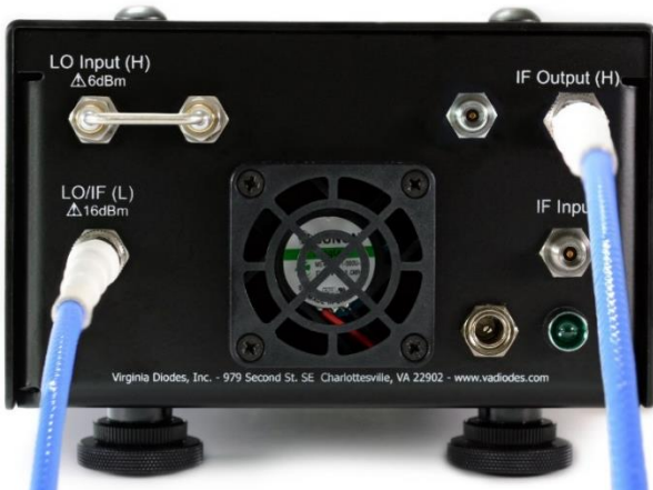
Figure 2: Block Down-Conversion – Low Frequency LO Input
