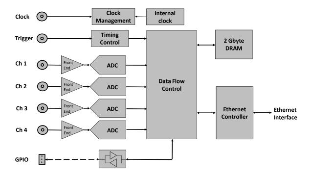
Figure 1: Block diagram 4-channel mode
